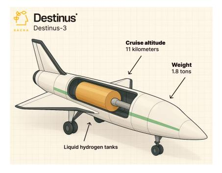
Destinus is building autonomous hypersonic aircraft—called hyperplanes—that can travel at five times the speed of sound (Mach 5+) using liquid hydrogen as fuel. These aircraft take off from conventional runways like normal planes, climb to near-space altitudes (30-60km), accelerate to hypersonic speeds using a two-stage propulsion system, and then glide toward their destination before landing on standard airports—all while producing zero carbon emissions, with water vapor as the only exhaust.
